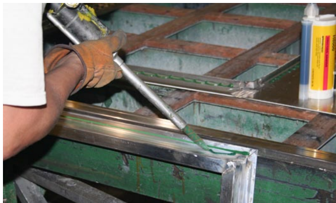
Loctite® H8000™ is used to bond the ambulance bodies' aluminum skin to frame members. The process is quick and economical.
